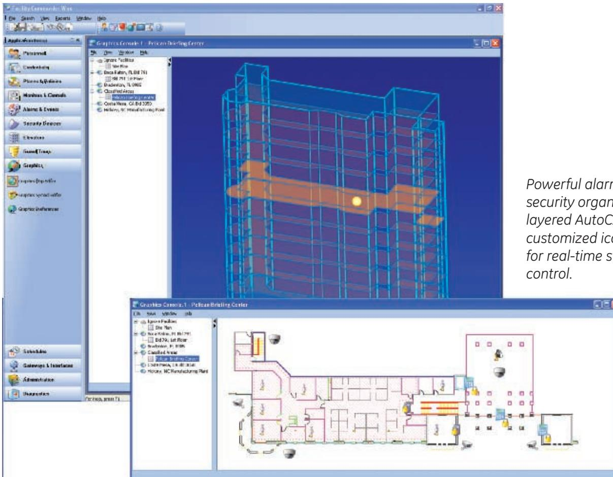
*Powerful alarm graphics allow your security organization to import multi-layered AutoCAD drawings and customized icons to represent devices for real-time status monitoring and control.*
